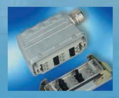
The Modular system enables signal and power contacts within one connector housing and provides flexibility to adapt connector configurations to individual customer needs. Every user can select their own connection designs with up to 280 contacts in a single housing. The series also offers many coding possibilities.
