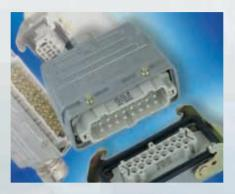
The universal series C146E provides 6 to 24 contacts in screw or crimp termination. The crimp contacts are available as turned or stamped versions. Also offered is a "Double Density" option with up to 48 turned crimp contacts.
