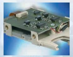
The manual Hybrid Reader accepts magstripe cards and smart cards in the same slot. There is no need to change the connector in case of switching the card system. Cards can be substituted gradually without a loss in convenience for the user. Due to compact design the Hybrid Reader can be integrated in existing systems easily. Smart card reader features landing contacts.
