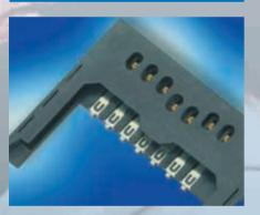
Along with the MultiMediaCard- and Secure Digital (SD) Card Connectors we also offer contact solutions for half size and high speed MultiMediaCards as well as combined solutions. The emphasis of development is therefore compact dimensions and automated assembly.
